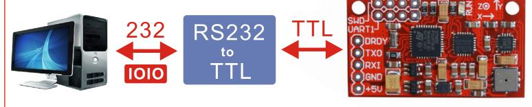
RS232 to TTL level adapter to connect
