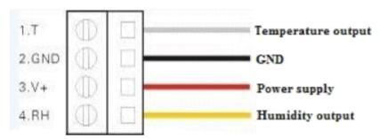
(2). Connection Diagram for current output
