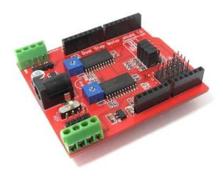
Dual stepper motor driver shield can drive 2 stepper motors at the same time by Arduino. It can work with the power supply from 4.75V to 30V. High accuracy controlling can be supported by Arduino for CNC milling machine.
