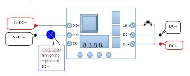
Gentle remind: If user load and FRMO1 module use a seam DC power supply, it is possible because of the power supply capacity is insufficient or wiring connections unfit, the module appears unstable phenomenon occasionally, please use the following (even if no found the problem, it should follow the recommendations):
