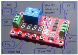
Keys include long press and short press, and in different modes with different functions, the following is to introduce under three mode key's different functions.
